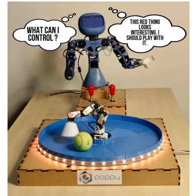
Figure 2.17: An intrinsically motivated agent learns what effects can be produced by its action and uses it to explore its environment leading to nested tool use discovery [58]
